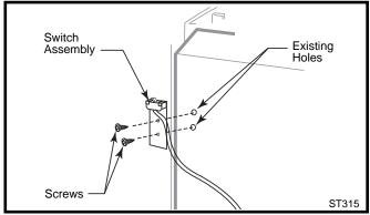
Fig. 40 Attach switch assembly to rear shroud.
